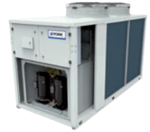
YLZ Air to water HP E.V.I 4 pipe system Scroll E.V.I Com. / R410A Hot water up to 65°C Heating capacity: 25 to 210 kW
