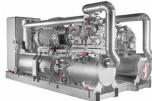
DualPAC recip 2-stages Variable-Speed Drive Reciprocating compr. / R717 Hot water up to 70°C Heating cap. 400 to 3000 kW Hot water up to 90°C (HPX) Heating cap. up to 1850 kW
