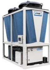
YMPA Air to water HP Scroll compr. / R410A Hot water up to 55°C Heating capacity: 50 to 254 kW
