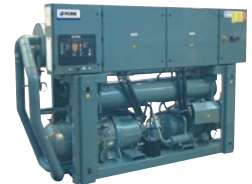
YLCS Water to water HP Twin screw / R134a (R513A on request) Hot water up to 65°C Heating capacity: 440 to 990 kW
