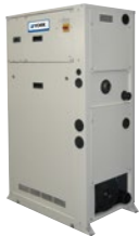
YMWA Water to water HP Scroll compr. / R410A Hot water up to 55°C Heating capacity: 24 to 212 kW
