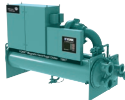
YMC² Water to water heat pump VSD Centrifugal compr. Mag. bearings / R134a & R513A Hot water up to 50°C Heating cap.: 900 to 4,000 kW
