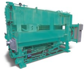
YHAP Single stage absorption Steam, Gas or Hot Water driven / R718 Hot water up to 95°C Heating cap.: 900 to 40,000 kW
