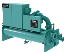
YMC² Water to water heat pump Variable speed centrif. compr. Magnetic bearings / R134a & R513A Hot water up to 65°C Heating cap.: 1600 to 3000 kW
