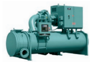
YK HP Water to water heat pump Centrifugal compr. / R134a Hot water up to 50°C (Std) Hot water up to 70°C (HP) Heating cap.: 1000 to 9000 kW
