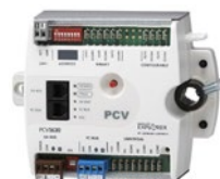
FX-PCV1630-1 Regulator with 8 physical points; 3UI, 3BO, 2CO; Integrated 4 Nm transducer and motor, 24 V AC power supply
