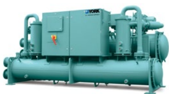
YVWA Water to water heat pump Screw compr. / R134a & R513A Hot water up to 63°C Heating cap.: 600 to 1000 kW
