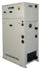
YMWA Water to water HP Scroll compressor / R410A Hot water up to 55°C Heating capacity: 24 to 212 kW
