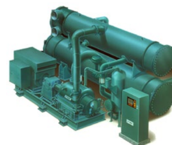
Titan OM HP Water to water heat pump Multi-stage Centrifugal, electric, steam or gas driven / R134a Hot water up to 90°C Heating capacity from 5000 to 20000 kW
