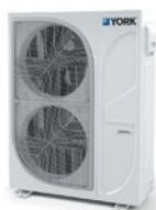
YVAG Air to water HP Scroll compressor / R410A Hot water up to 52°C Heating capacity: 10.9 to 18.4 kW
