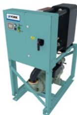
YCSE Water to water HP Screw compressor / R134a Hot water up to 55°C Heating capacity: 170 to 300 kW
