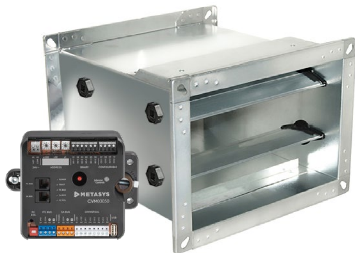
FX-PCV1630-1 Regulator with 8 physical points; 3UI, 3BO, 2CO; Integrated 4 Nm transducer and motor, 24 V AC power supply
