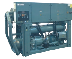
YLCS Water to water HP Twin screw / R134a Hot water up to 65°C Heating capacity: 440 to 990 kW
