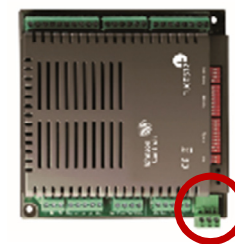
Fankoils... n Terminal Unit kontrolieris TUC0312-2
