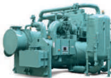
CYK HP Water to water heat pump Dual-Centrifugal compressors, Series-Arrangement / R134a Hot water up to 70°C Heating capacity from 2500 to 7000 kW
