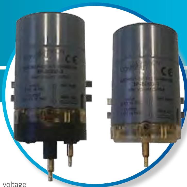
EP-8000 series electro-pneumatic transducers convert a voltage or current signal from an electronic controller into a pneumatic output pressure signal. An increase or decrease in the input signal proportionally increases or decreases (respectively) the output pressure signal from the EP-8000.
