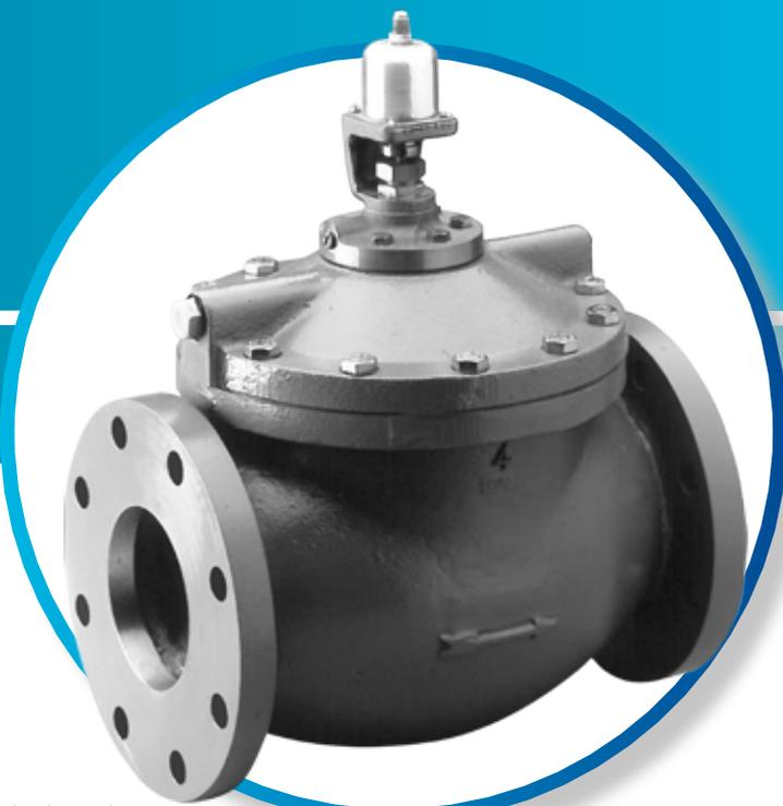
The V43 / V243 pressure-actuated water-regulating valves are designed to regulate water flow through the condenser of large refrigerated cooling systems. These pilot-operated valves open on an increase in refrigerant head pressure and provide modulating operation.
