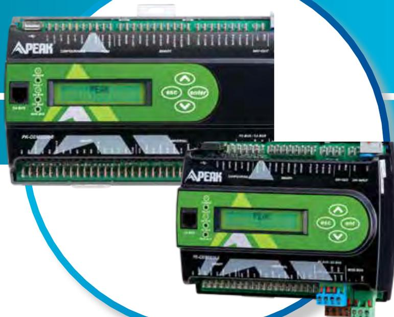
The PEAK 18 and PEAK 32 Controllers are configurable controllers that can be switched between MS/TP, Modbus® RTU, and N2 Communication protocols real-time through the onboard local display or through the Mobile Access Portal (MAP) Gateway. When the controllers are used as MS/TP devices, they are BACnet® Advanced Application Controllers (B-AACs) with integral RS-485 Master-Slave/Token-Passing (MS/TP) communications.
