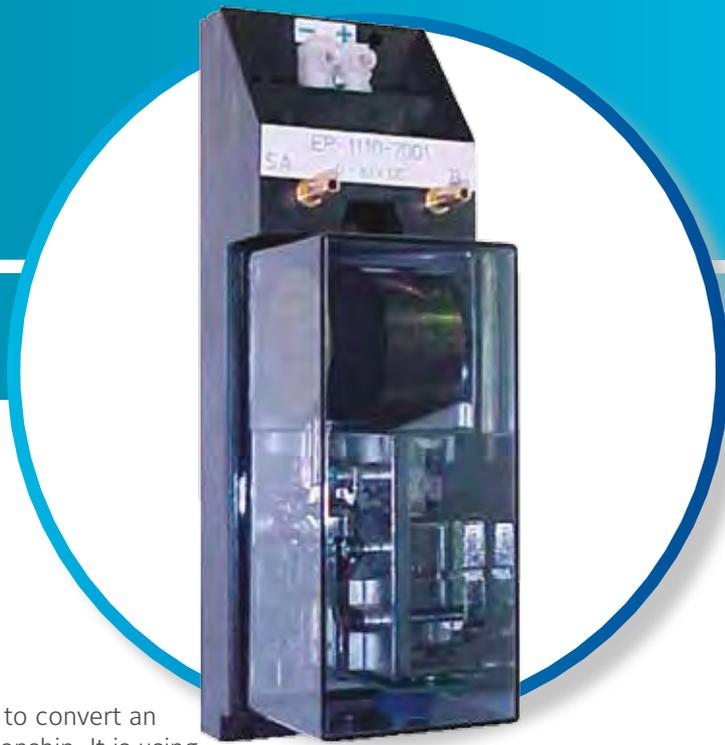
The EP-1110 is an electric to air pressure transducer designed to convert an electrical input signal into a pressure output with a linear relationship. It is using a force balance with moving coil system.
