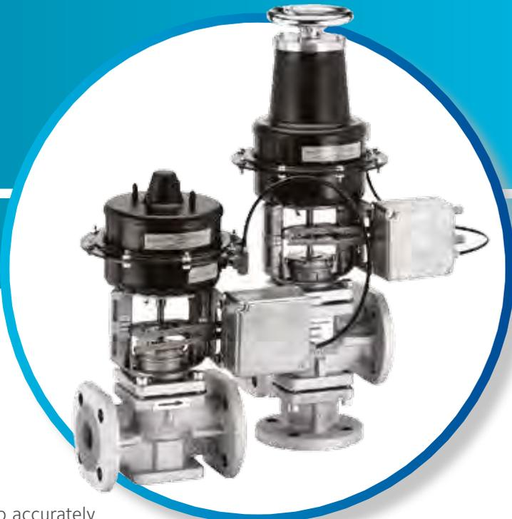
The MP8000 Series Pneumatic Valve-Actuators are designed to accurately position valve plugs in larger chilled water, hot water and steam applications in response to a pneumatic signal from a controller. A pneumatic positioner is also available for use in applications where sequential operation is desired or more positioning power and accuracy are required. They can be ordered as a factory fitted and ready-to-install valve/actuator combination or separately for local installation.
