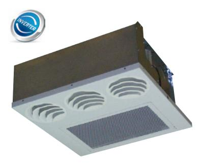
Thanks to its unique diffuser, YFCC cassette units generate an airflow with a "coanda" effect. The unit is suitable for installation in a suspended ceiling. Air intake is from the bottom while the air is supplied parallel to the ceiling.
