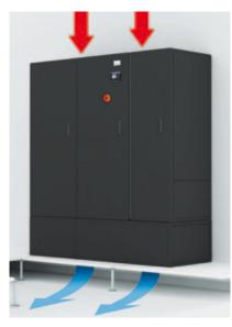
Version for perimetral installation inside the Data Centre with raised floor height less than 550 mm. In this case, the plinth with fixed height of 550 mm is supplied with lateral closure panels and must be installed above the floor. It is essential to check that the height of the ceiling is sufficient to ensure good air suction.
