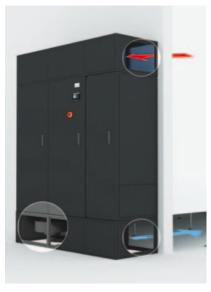
Version for installation outside the Data Centre, without raised floor, rear air supply. In this case the plinth (fixed height 550 mm) is supplied with side closure panels and rear supply air grilles. Installation of the plenum with rear re-intake system is optional, if there is no ductwork.
