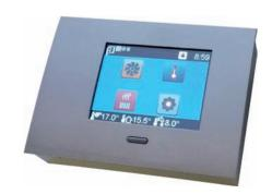
**Dimensions of the controller:** 125 mm long x 90 mm high x 32 mm deep
